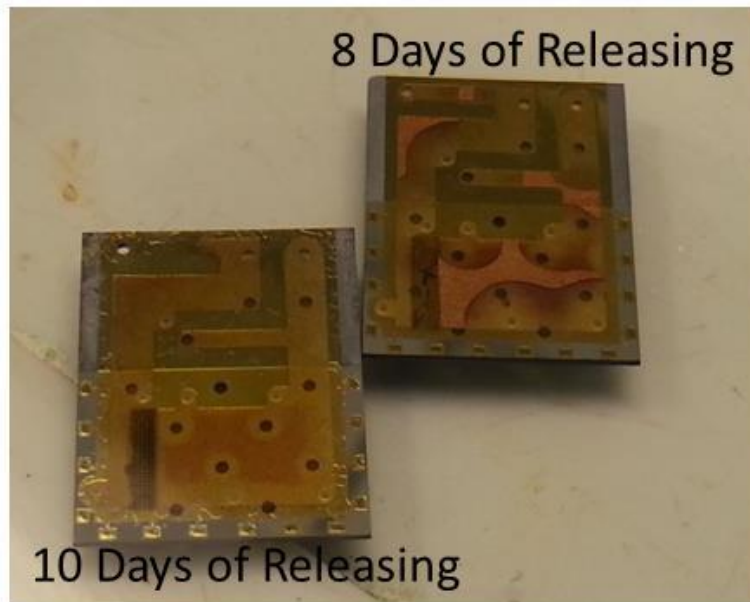
Figure 2.24: Two coldstage chips during the release process. One is fully released after 10 days and the other still has copper remaining inside the channel structure after 8 days.
