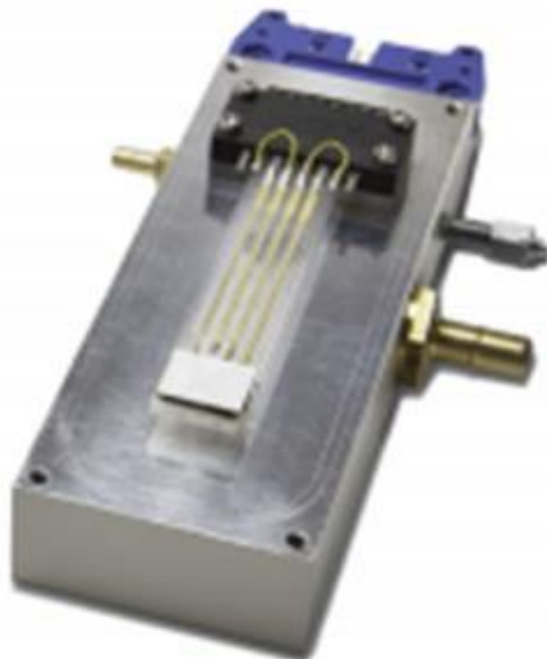
Figure 1.4: MMR Technologies microminiature refrigerator mounted to a vacuum flange [17].
