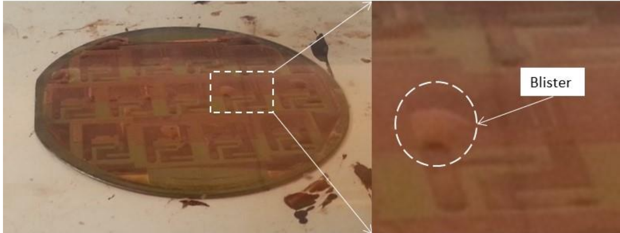
Figure 2.26: Wafer during second polyimide layer curing. Polyimide blisters formed when the wafer exceeded 200 °C
