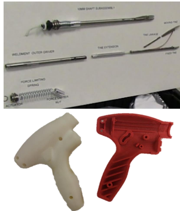
Figure 22. Prototypes of the benchmarked surgical device components (top) and two different material handle halves created in parallel (bottom) from the Medical Device Company
