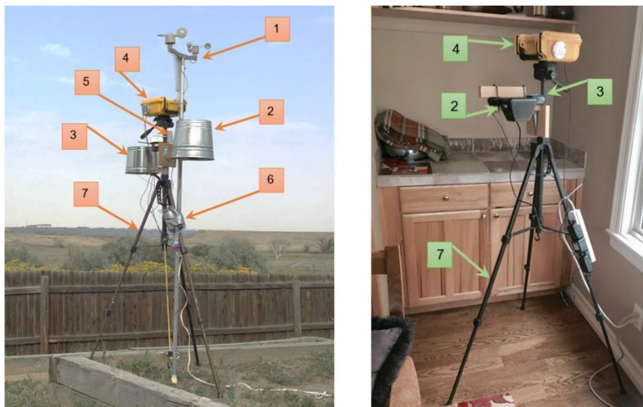
Figure S4. 1 Outdoor instrument rig (Left) and Indoor Instrument rig (Right). [Legend for labels: 1=Weather station; 2= Dylos- 1700 Monitor (outdoor instrument covered with metallic bucket); 3=microAeth AE51 Aethalometer (outdoor instrument covered with metallic bucket); 4=Y-pod; 5=Ogawa NO 2 passive sampler; 6=weather-protected electrical connection point; 7=tripod stand.]
