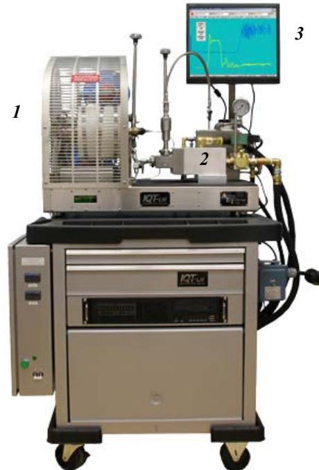
Figure 5: Ignition Quality Tester device, with 3 main components. 1: Combustion chamber. 2: Fuel delivery system. 3: Computer/software controls [34].
