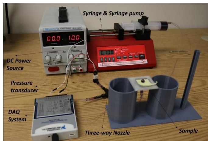
Fig.3-14. Picture of the testing system for VHB tape
