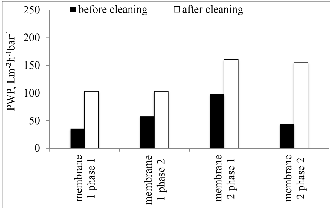
Figure 6.4 – Cleaning of the membrane module. Initial permeance of membrane 1 was 115 \text{ Lm}^{-2}\text{h}^{-1}\text{bar}^{-1} and membrane 2 was 175 \text{ Lm}^{-2}\text{h}^{-1}\text{bar}^{-1} .
