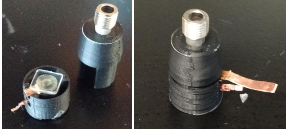
Figure 4-7 The 3D printed microendoscope design. The capsule includes two fixed glass lenses and the electrowetting lens encased with copper electrodes and the fiber optic coupler.
