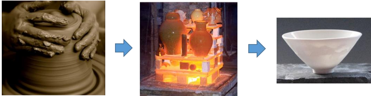
Figure 2.1 Clay body being given shape on a wheel and fired at high temperature to give final product, that is, a porcelain bowl. [12] .
