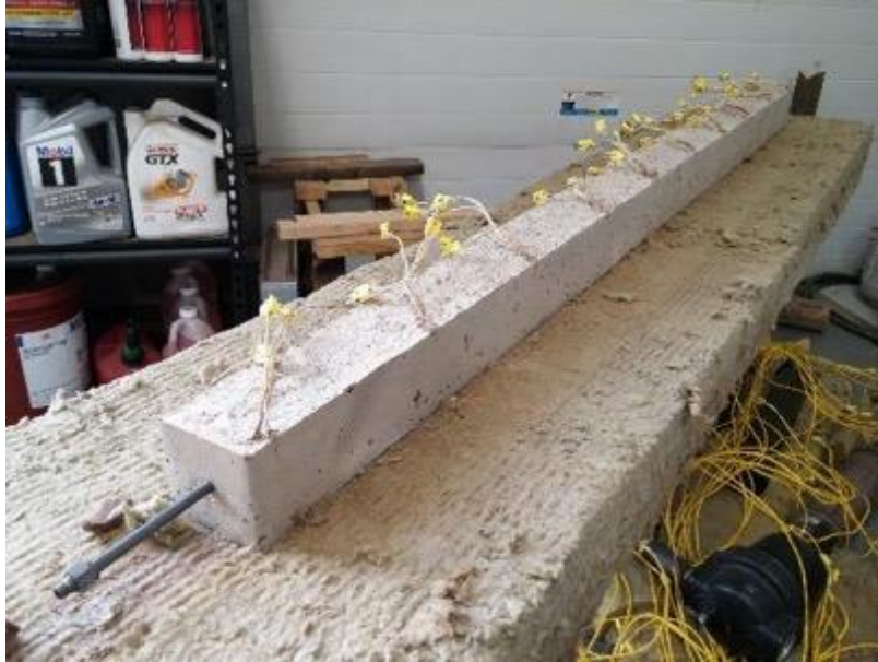
Figure 10: Picture of the tube-in-concrete test specimen before being wrapped in insulation.
