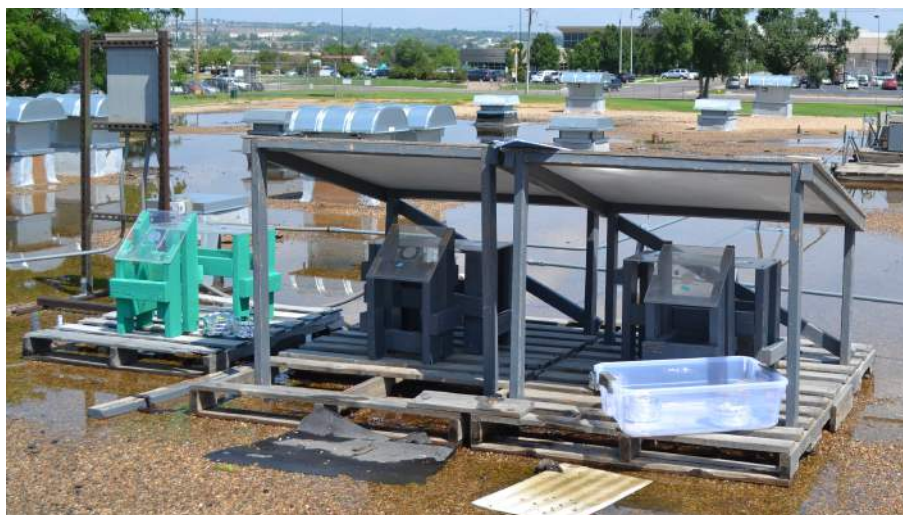
Figure 6.1: The three sample deployment structures used at the Commerce City site. The two on the right have roofs to prevent wet deposition of particles and cleaning by precipitation and represent the duplicate set-ups, while the one on the left does not have a roof, and is used for assessment of the impact of precipitation
