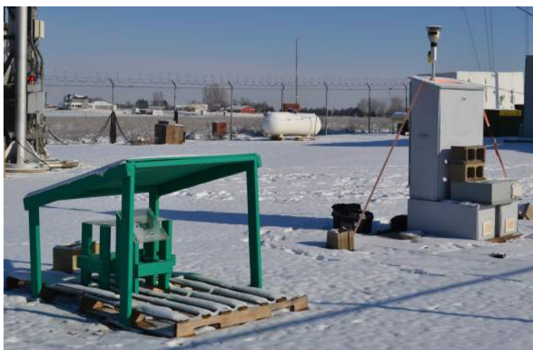
Figure 4.1: The experimental set-up at the Erie site. On the left is the deposition set-up, and on the right is the dichotomous filter sampler
