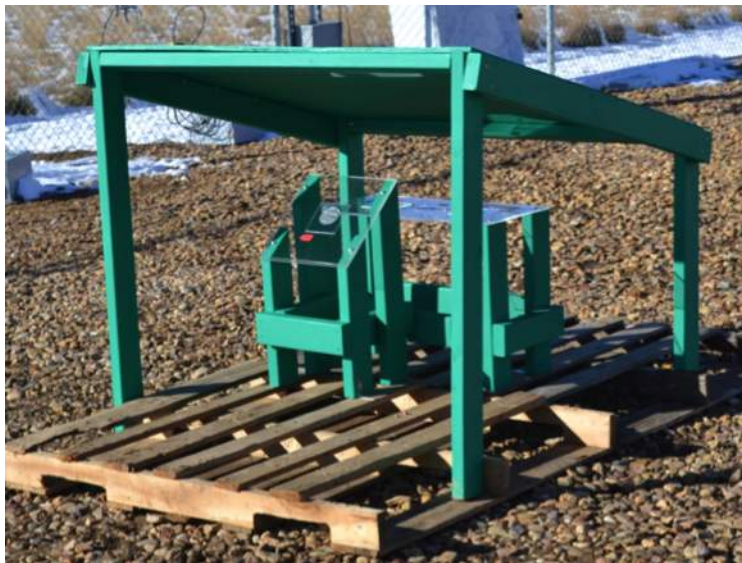
Figure 3.1: Set-up used for the deployment of PV cover plates in this study. This is at the Erie site, the Commerce City site used two nearly identical set-ups placed side by side.
