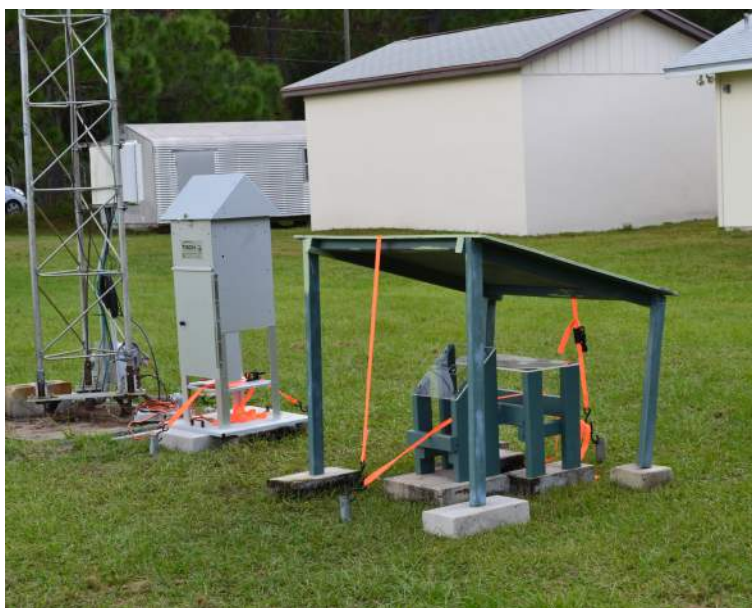
Figure 5.2: Set-up used for collection of samples at the Cocoa, Florida field site. On the left is the TSP filter sampler, and on the right is the deposition coupon deployment structure.
