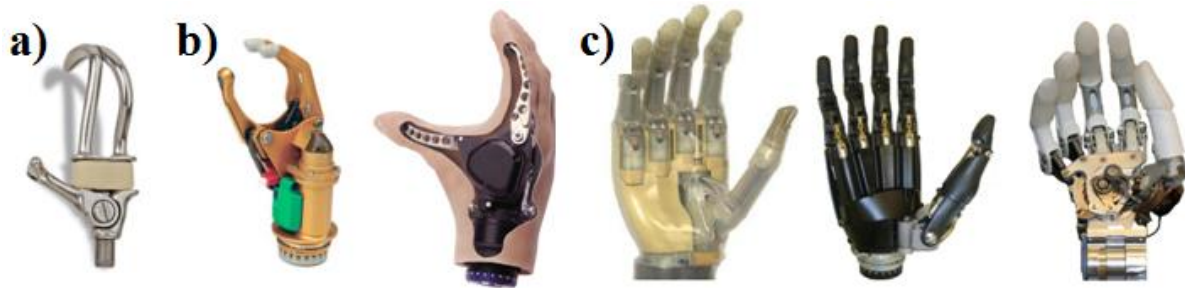
Figure 2. – Examples of (a) body-powered (b) single degree of actuation and (c) multifunction prosthetic hands. The hands shown are the Hosmer Hook, the Otto Bock MyoHand VariPlus Speed, the Motion Control ProControl hand, the Touch Bionics iLimb hand, the RSL Steeper Bebionic hand, and the Otto Bock Michelangelo hand respectively.
