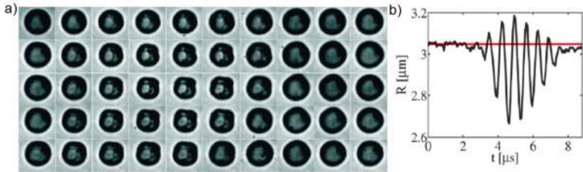
Figure 1.5 (a) High-speed optical micrographs of microbubble oscillations displaying a buckled shell during compression. (b) The corresponding radius-time curve where the “compression-only” behavior is apparent (from Sijl et. al. ) [15].
