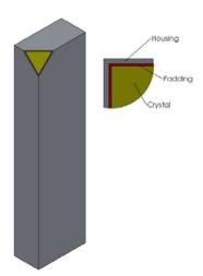
Figure 22: St. Gobain 16"x4"x2" NaI Detector (produced by Holmes)
