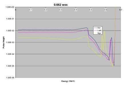
Figure 32: Without Heath can, different types of 3x3 Detectors for 0.662 MeV
