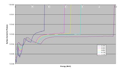
Figure 11: Photon spectrum incident on the crystal after being attenuated thought the can.
