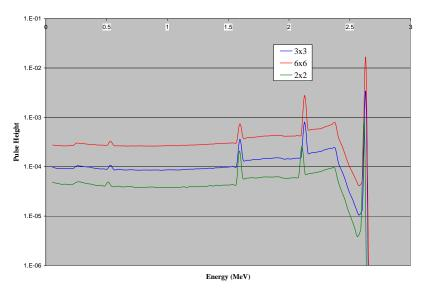
Figure 31: Heath can for different size NaI detectors With Detector Housing (Can) for  $2.614 \; \text{MeV}$
