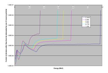
Figure 21: Photon spectrum incident on the crystal after being attenuated thought the can
