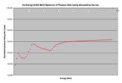
Figure 24: Cesium spectra point wise after attenuated through the front of the protective
