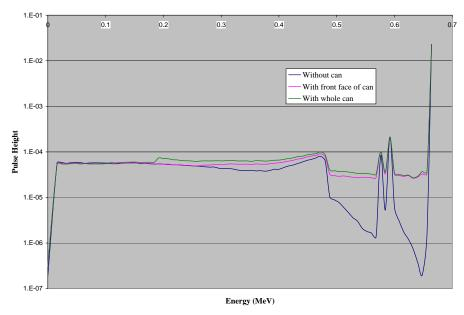
Figure 42: 3x3 BGO detectors at 0.662 incident energy
