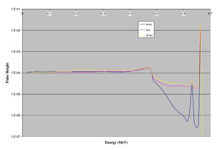
Figure 38: 3x3 LaBr detectors at 0.662 incident energy 256 channels with Heath can
