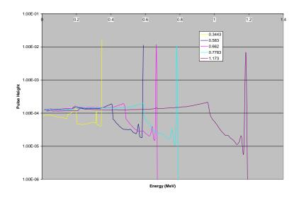
Figure 1: Part of an MCNP detector unspread response function for Sodium Iodide (NaI)
