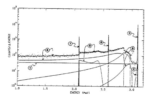
Figure 2: Components of the detector response function for Ge Detector (1) the flat continuum, (2) the exponential tail, (3) the full energy peak, (4) the Compton electron scattering continuum, (5) a continuum between the Compton electron scattering continuum and the full energy peak, (6) the single escape peak, (7) the double escape peak, (8) a small scattering continuum between the single and double escape peaks (Y. Jin, R. P. Gardner, and K. Verghese, 1986).
