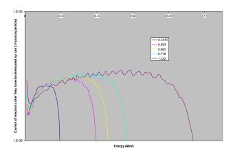
Figure 20: Electron spectrum incident on the crystal after being attenuated thought the can.
