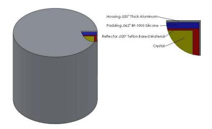
Figure 23: Typical Detector Housing for all produced 2x2 Cylindrical Detector (produced by Holmes)
