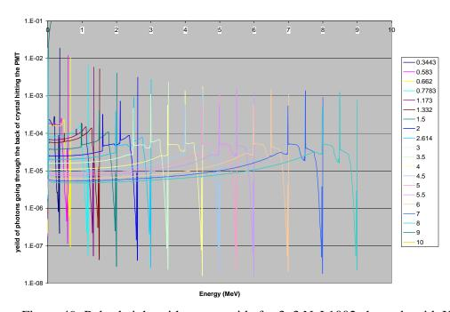
Figure 49: Pulse height with out can side for 3x3 NaI 1002 channels with Heath can
