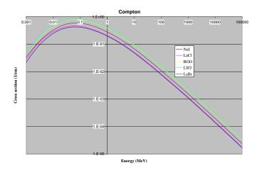
Figure 6: Compton (Incoherent) Scattering Cross Sections for many types of detectors.
