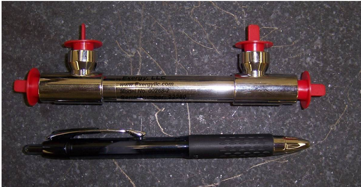
Figure 12: Exergy LLC model 00268-2 shell and tube heat exchanger
