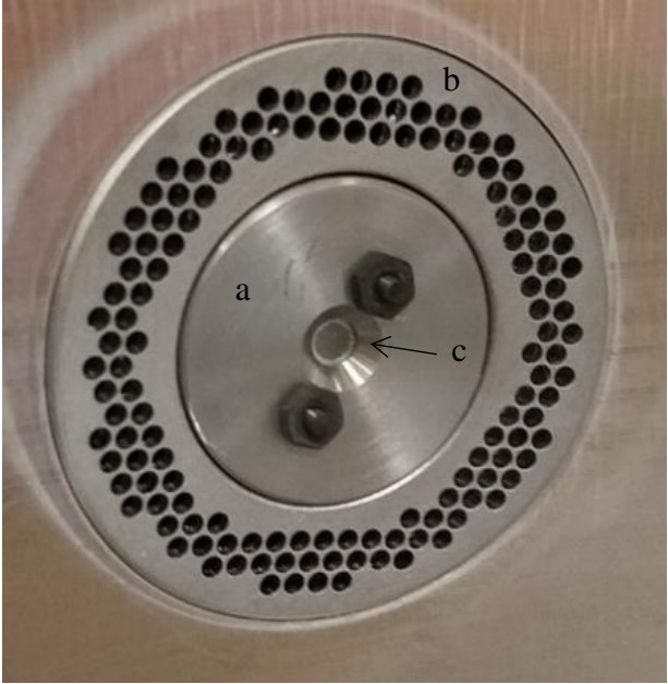
Fig. 75: Pictures of the TEL RFEA wall probe (WP). (Left) Picture of the front of the grid in the wall of the chamber (a) Ground cover that covers the probe and attaches to the differential pumping shaft (b) Port cover to prevent light-up down the outside of the differential pumping shaft (c) Floating (1 st ) grid (Right) Picture of the WP housing on the outside of the chamber (a) Linear stage that moves the probe in and out of the chamber (b) differential pumping line (c) Bellows that covers the differential pumping shaft on which the RFEA is mounted.
