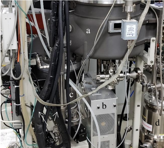
Fig. 34: Pictures of the TEL 200mm DRM chamber. (a) 200mm DRM chamber housing (b) 13MHz matching network (c) Main chamber turbomolecular pump (d) Diagnostic differential turbomolecular pump (e) Feedthrough for RFEAs in the bottom electrode (f) Bottom electrode cooling lines.
