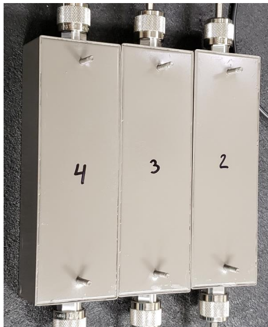
Fig. 96: Picture of the Allen Avionics filters attached to one of the electrode RFEA probes.
