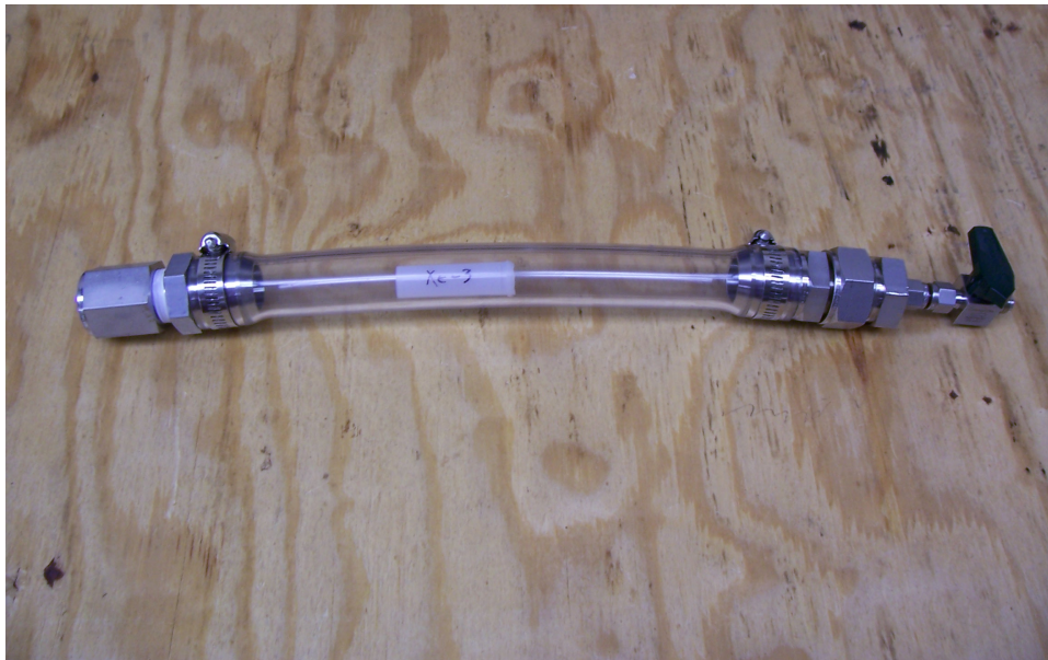
Fig. A.4 Radioactive Sample Transfer device with Xe-3 sample inside
