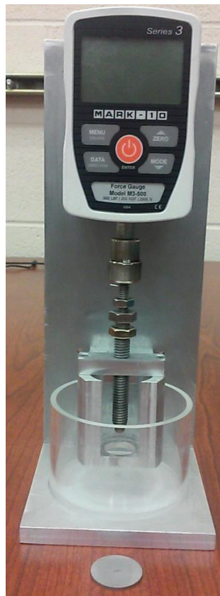
Figure 9-1: Experimental apparatus for constant load testing of SCC
