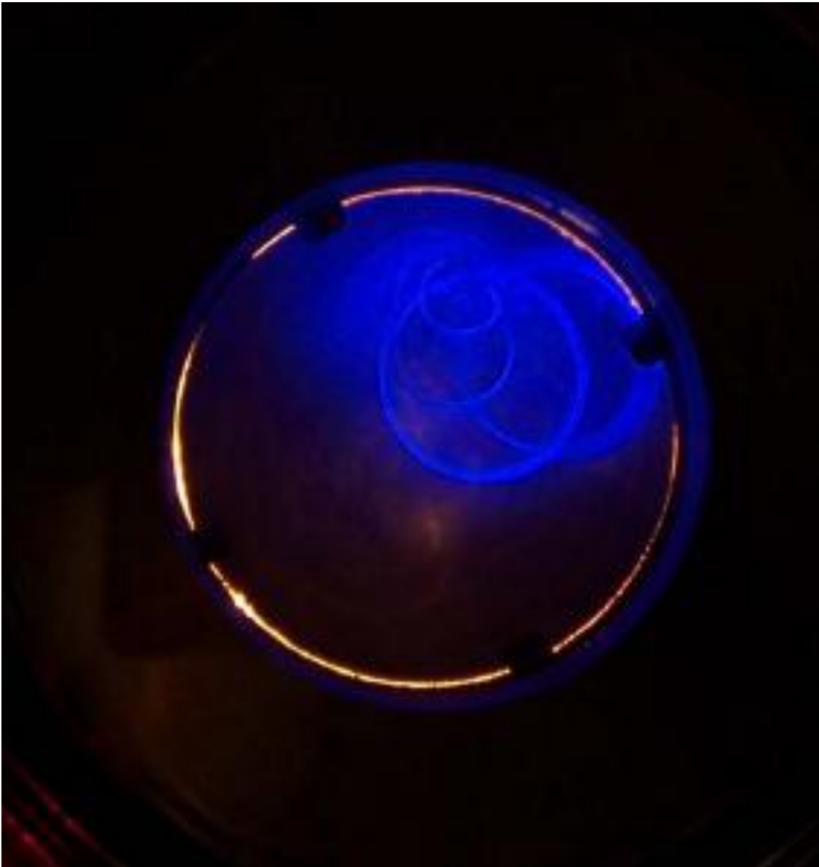
Fig. 3.2. Image demonstrating the effectiveness of the extraction optics of the slow positron beam using electron guns and phosphor screen.
