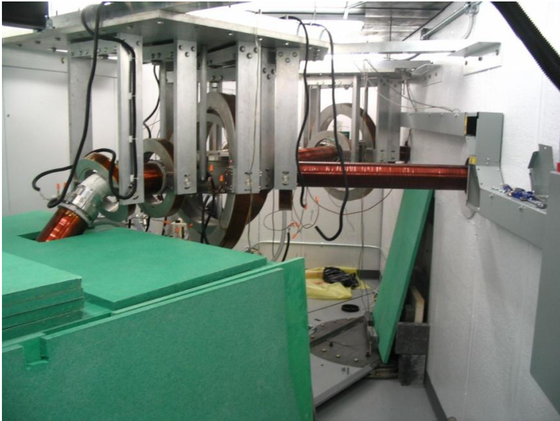
Fig. 3.10. Image of the assembled coils used to magnetically guide positrons into the respective labs
