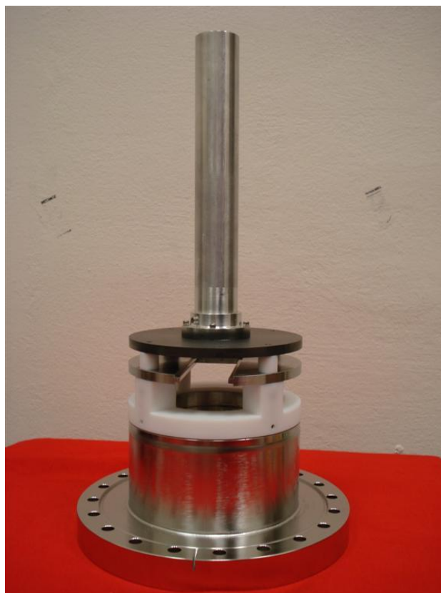
Fig. 4.22. Image of the sample holder and accompanying drift lens. The lens stack is attached to the detector well of the vacuum chamber using a Teflon holder.
