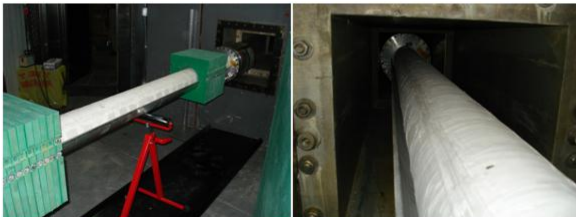
Fig. 3.8. Images of insertion of the slow positron beam into beam tube 6.
