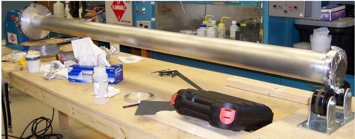
Fig. 2.27. Image of the solenoid vacuum chamber mounted on welding positioning head prior to winding the solenoid.
