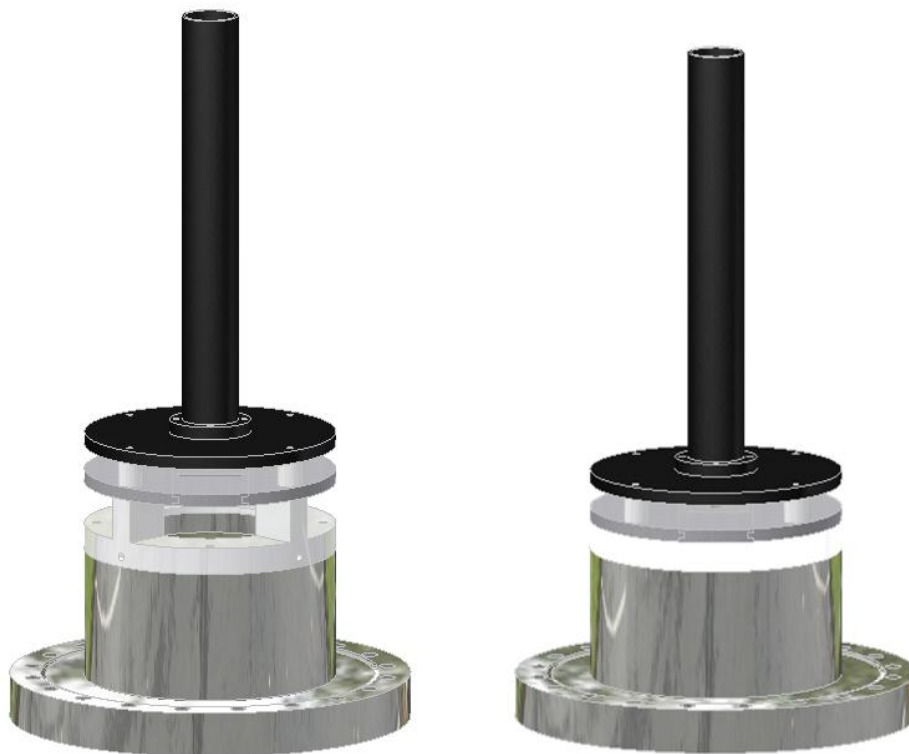
Fig. 5.5. Image of the current target stage of the spectrometer (Left) compared to a modified moderator stage (right) with an expected detection efficiency of 0.21%.
