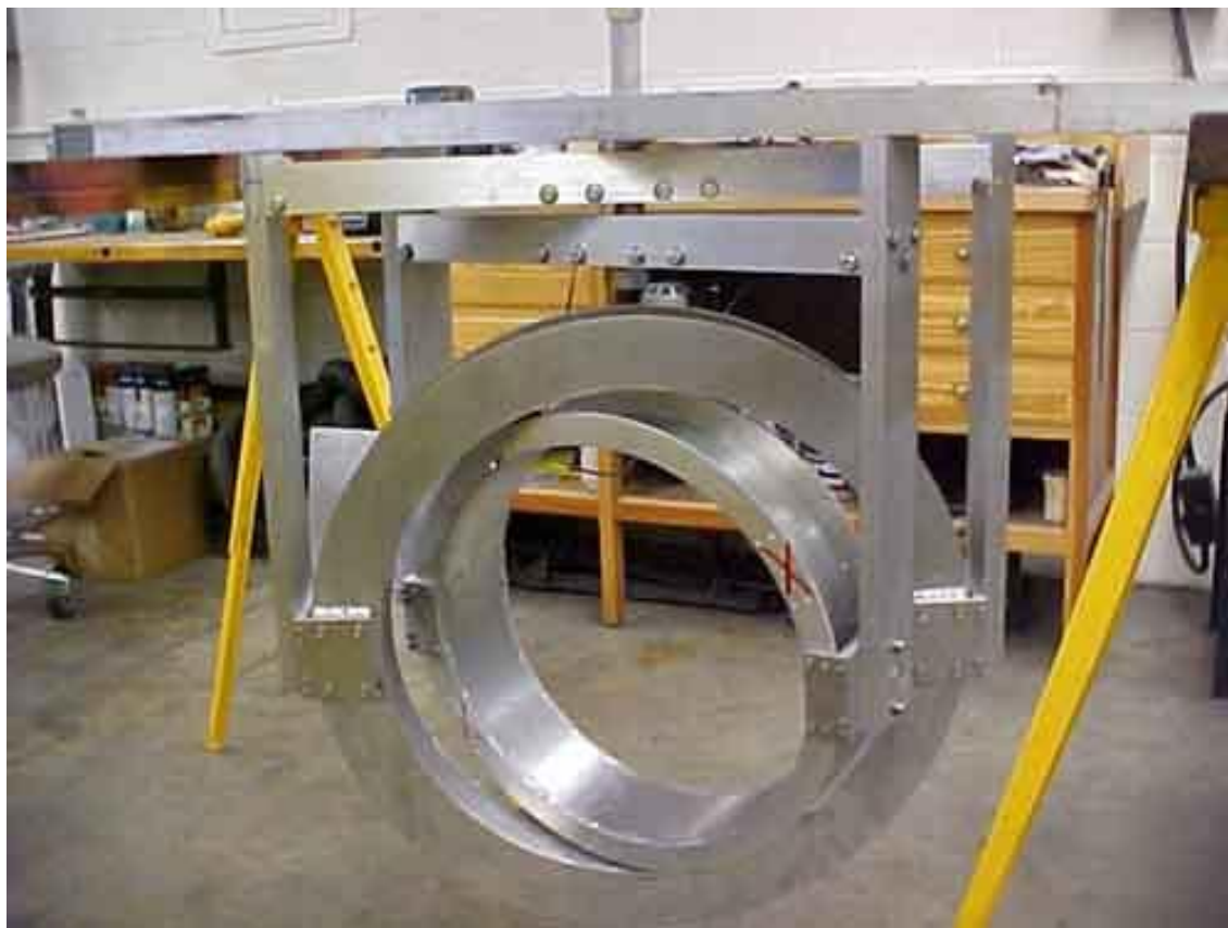
Fig. 2.30. Image of the gimbal and coil forms used to guide positrons through the first switchyard. c
