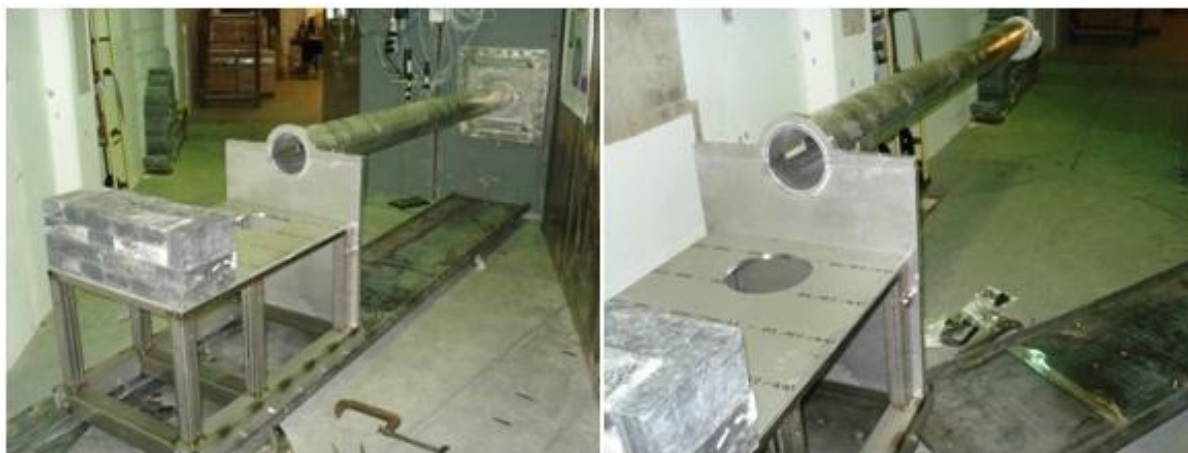
Fig. 2.32. Image of the cart and track used to support and guide the slow positron beam into beam tube 6 of the PULSTAR reactor.
