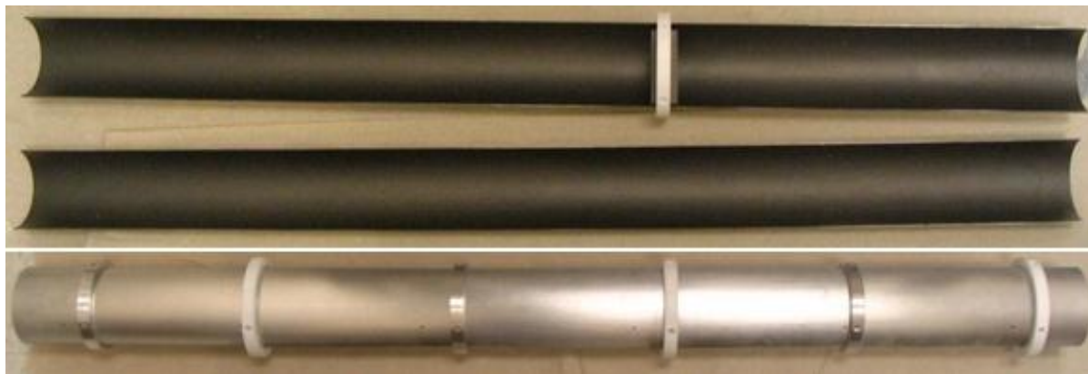
Fig. 4.17. Image of the drift lens for the pulsed positron spectrometer. The lens is cut in half and reassembled to allow the application of graphite to the internal surface and the installation of the internal shield.
