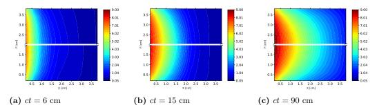
**Figure 3.36** Total energy density  $(E \times 10^{-13} \frac{erg}{cm^3})$  computed by the multi-level QD method using the MSCB transport scheme with  $\tau = 2 \times 10^{-3}$ sh using (i) the monotonized hybrid method (top-half) and (ii) the hybrid method (bottom-half) on a 10x10 mesh.
