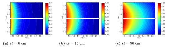
**Figure 3.32** Total energy density  $(E \times 10^{-13} \frac{erg}{cm^3})$  computed by the multi-level QD method using the MSCB transport scheme with  $\tau = 2 \times 10^{-3}$ sh using (i) the first order method (top-half) and (ii) the hybrid method (bottom-half) on a 10x10 mesh.
