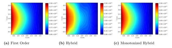
**Figure 3.40** Energy Density (in  $E \times 10^{-13} \frac{erg}{cm^3}$ ) computed with  $\tau = 2 \times 10^{-3}$ sh by the multi-level QD method in Group 13 using the MSCB transport scheme on a 10x10 mesh.
