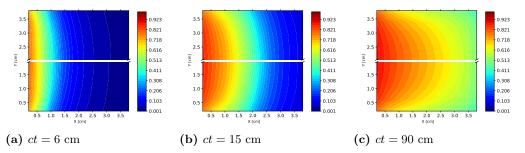
Figure 3.2 Temperature (in keV) computed by the multi-level QD method using the MSS transport scheme with  $\tau$ =2×10<sup>-3</sup>sh using (i) the first order method (top-half) and (ii) the hybrid method (bottom-half) on a 10x10 mesh.
