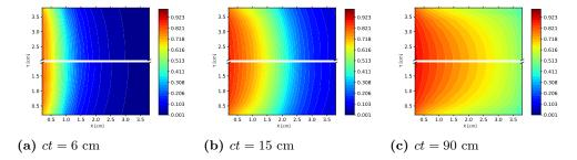
Figure 3.14 Temperature (in keV) computed by the multi-level QD method with using the MSS transport scheme  $\tau=2\times10^{-3}$ sh using (i) the monotonized hybrid method (top-half) and (ii) the hybrid method (bottom-half) on a 10x10 mesh.
