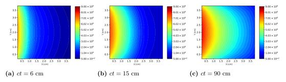
**Figure 3.50** Total energy density  $(E\times 10^{-13}\frac{erg}{cm^3})$  computed by the two-level  $P_1$  method using the backward-Euler scheme with  $\tau$ =2×10<sup>-3</sup>sh on a 10x10 mesh.
