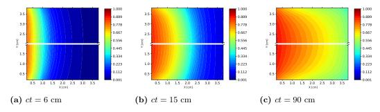
Figure 3.31 Temperature (in keV) computed by the multi-level QD method using the MSCB transport scheme with  $\tau=2\times10^{-3}$ sh using (i) the first order method (top-half) and (ii) the hybrid method (bottom-half) on a 10x10 mesh.
