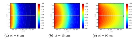
Figure 3.18 Temperature (in keV) computed by the multi-level QD method with using the MSS transport scheme  $\tau=2\times10^{-3}$ sh using (i) the monotonized hybrid method (top-half) and (ii) the hybrid method (bottom-half) on a 20x20 mesh.
