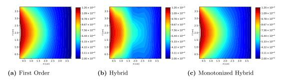
**Figure 3.41** Energy Density (in  $E \times 10^{-13} \frac{erg}{cm^3}$ ) computed with  $\tau = 2 \times 10^{-3}$ sh by the multi-level QD method in Group 16 using the MSCB transport scheme on a 10x10 mesh.
