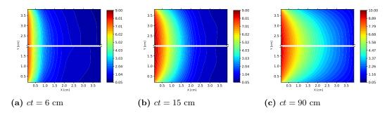
**Figure 3.8** Total energy density  $(E \times 10^{-13} \frac{erg}{cm^3})$  computed by the multi-level QD method using the MSS transport scheme with  $\tau = 2 \times 10^{-3}$ sh using (i) the first order method (top-half) and (ii) the hybrid method (bottom-half) on a 20x20 mesh.
