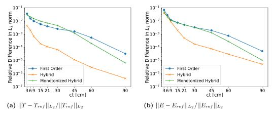
Figure 3.29 The relative difference of the solution obtained by the multi-level QD method using the MSS transport scheme compared to the reference solution in the  $L_2$  norm,  $\tau = 2 \times 10^{-3}$  sh on a 10x10 mesh.
