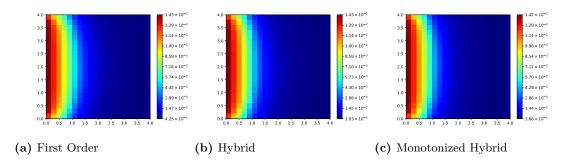
**Figure 3.21** Cell-averaged values of the energy density (in  $E \times 10^{-13} \frac{erg}{cm^3}$ ) computed with  $\tau = 2 \times 10^{-3}$ sh by the multi-level QD method using the MSS transport scheme in Group 1 on a 20x20 mesh.
