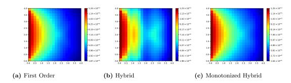
**Figure 3.25** Cell-averaged values of the energy density (in  $E \times 10^{-13} \frac{erg}{cm^3}$ ) computed with  $\tau = 2 \times 10^{-3}$ sh by the multi-level QD method using the MSS transport scheme in Group 16 on a 20x20 mesh.
