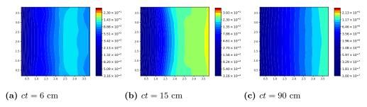
Figure 3.16 Relative difference in temperature computed by the multi-level QD method using the MSS transport scheme with  $\tau=2\times10^{-3}$ sh using (i) the monotonized hybrid method (top-half) and (ii) the hybrid method (bottom-half) on a 10x10 mesh.
