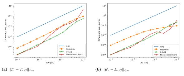
Figure 3.30 Convergence study at ct=6cm in the  $L_{\infty}$  norm for the solution obtained by the multilevel QD method using the MSS transport scheme on a 10x10 mesh.
