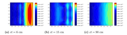
**Figure 3.11** Relative difference in total energy density  $(E \times 10^{-13} \frac{erg}{cm^3})$  computed by the multi-level QD method using the MSS transport scheme with  $\tau = 2 \times 10^{-3}$ sh using (i) the first order method (tophalf) and (ii) the hybrid method (bottom-half) on a 10x10 mesh.
