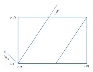
Figure 2.1 Subcells formed by a particular streaming direction and the local coordinate system for the first triangle subcell in cell (ij).
