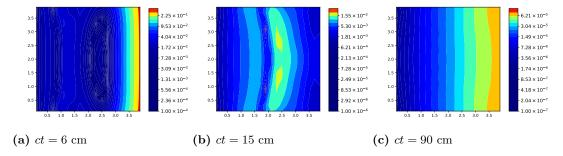
Figure 3.12 Relative difference in temperature computed by the multi-level QD method using the MSS transport scheme with  $\tau=2\times10^{-3}$ sh using (i) the first order method (top-half) and (ii) the hybrid method (bottom-half) on 20x20 mesh.
