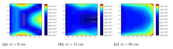
Figure 4.18 Relative difference in the energy density computed with  $\tau=2\times10^{-3}$  sh by the multilevel QD method using the RT equation with the Minerbo closure and the first-order scheme.
