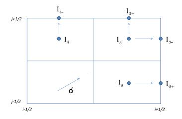
Figure 2.3 Upwinding condition for SCB scheme.
