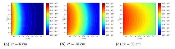
Figure 3.49 Temperature (in keV) computed by the two-level  $P_1$  method using the backward-Euler scheme with  $\tau=2\times10^{-3}$ sh on a 10x10 mesh.
