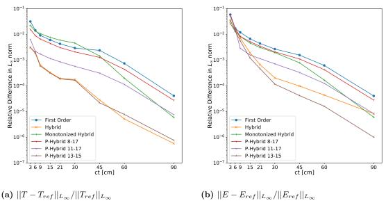
Figure 3.47 The relative difference between the solution at  $\tau=2\times10^{-3}$ sh and the reference solution in the  $L_{\infty}$  norm obtained by the multi-level QD method using the MSS transport scheme with P-Hybrid on a 10x10 mesh.
