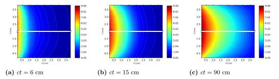
Figure 4.17 Energy density  $(E \times 10^{-13} \frac{erg}{cm^3})$  computed with  $\tau = 2 \times 10^{-3}$  sh by the QD method using (i) the first-order scheme (top half) and (ii) RT equation with the Minerbo closure (bottom half).
