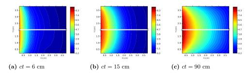
**Figure 3.15** Total energy density  $(E \times 10^{-13} \frac{erg}{cm^3})$  computed by the multi-level QD method using the MSS transport scheme with  $\tau = 2 \times 10^{-3}$ sh using (i) the monotonized hybrid method (top-half) and (ii) the hybrid method (bottom-half) on a 10x10 mesh.
