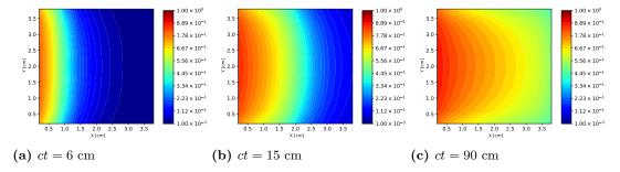
Figure 3.51 Temperature (in keV) computed by the two-level  $P_1$  methods using the Crank-Nicolson scheme with  $\tau=2\times10^{-3}$ sh on a 10x10 mesh.
