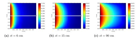
**Figure 3.9** Cell-averaged values of the total energy density  $(E \times 10^{-13} \frac{erg}{cm^3})$  computed by the multilevel QD method using the MSS transport scheme with  $\tau$ =2×10<sup>-3</sup>sh using (i) the first order method (top-half) and (ii) the hybrid method (bottom-half) on a 20x20 mesh.
