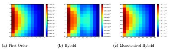
**Figure 3.24** Cell-averaged values of the energy density (in  $E \times 10^{-13} \frac{erg}{cm^3}$ ) computed with  $\tau = 2 \times 10^{-3}$ sh by the multi-level QD method using the MSS transport scheme in Group 16 on a 10x10 mesh.
