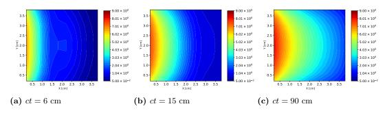
**Figure 3.52** Total energy density  $(E \times 10^{-13} \frac{erg}{cm^3})$  computed by the two-level  $P_1$  method using the Crank-Nicolson scheme with  $\tau = 2 \times 10^{-3}$ sh on a 10x10 mesh.
