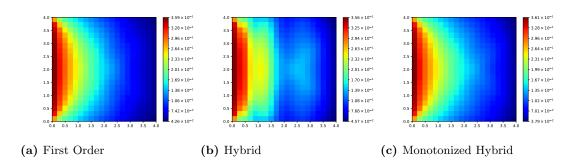
**Figure 3.23** Cell-averaged values of the energy density (in  $E \times 10^{-13} \frac{erg}{cm^3}$ ) computed with  $\tau = 2 \times 10^{-3}$ sh by the multi-level QD method using the MSS transport scheme in Group 13 on a 20x20 mesh.
