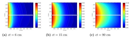
**Figure 3.19** Total energy density  $(E \times 10^{-13} \frac{erg}{cm^3})$  computed by the multi-level QD method using the MSS transport scheme with  $\tau = 2 \times 10^{-3}$ sh using (i) the monotonized hybrid method (top-half) and (ii) the hybrid method (bottom-half) on a 20x20 mesh.
