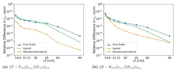
Figure 3.43 The relative difference between the solution at  $\tau$ =2×10<sup>-3</sup>sh and the reference solution in the  $L_{\infty}$  norm obtained by the multi-level QD method using the MSCB transport scheme on a 10x10 mesh.
