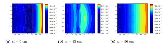
Figure 3.33 Relative difference in temperature computed by the multi-level QD method using the MSCB transport scheme with  $\tau=2\times10^{-3}$ sh using (i) the first-order method (top-half) and (ii) the hybrid method (bottom-half) on a 10x10 mesh.
