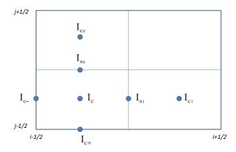
Figure 2.2 Cell unknowns of the SCB scheme.
