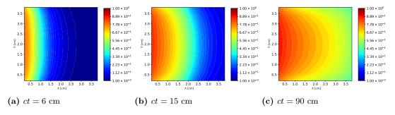
Figure 3.53 Temperature (in keV) computed by the two-level  $P_1$  method using the L-TRAP scheme with  $\tau=2\times10^{-3}$ sh on a 10x10 mesh.
