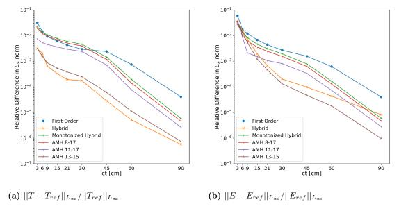
Figure 3.45 The relative difference between the solution at  $\tau=2\times10^{-3}$ sh and the reference solution in the  $L_{\infty}$  norm obtained by the multi-level QD method using the MSS transport scheme with AMH on a 10x10 mesh.
