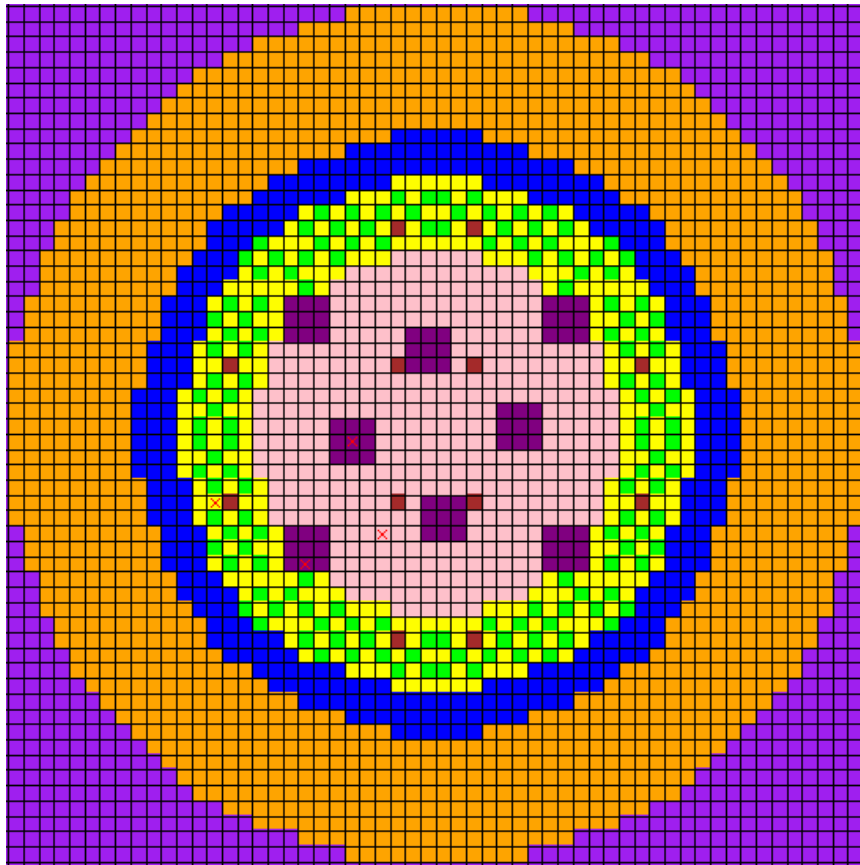
Figure 4.6 : ZPPR-15B with mock SNF assemblies.
