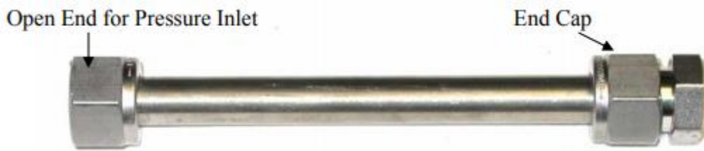
Figure 3.7. FeCrAl sample used for burst testing.
