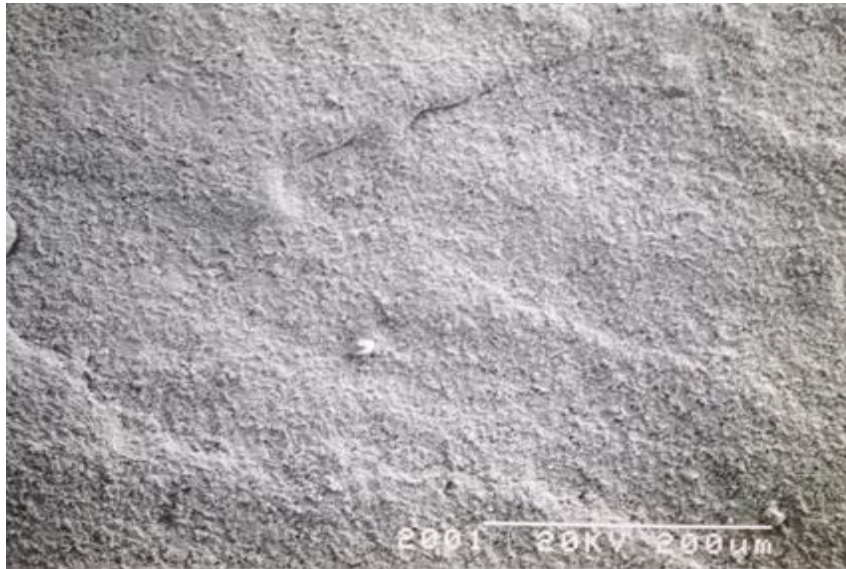
Figure 5.5: Photograph of steel surface after a 6 kJ ET discharge showing surface ablation due to direct sublimation.
