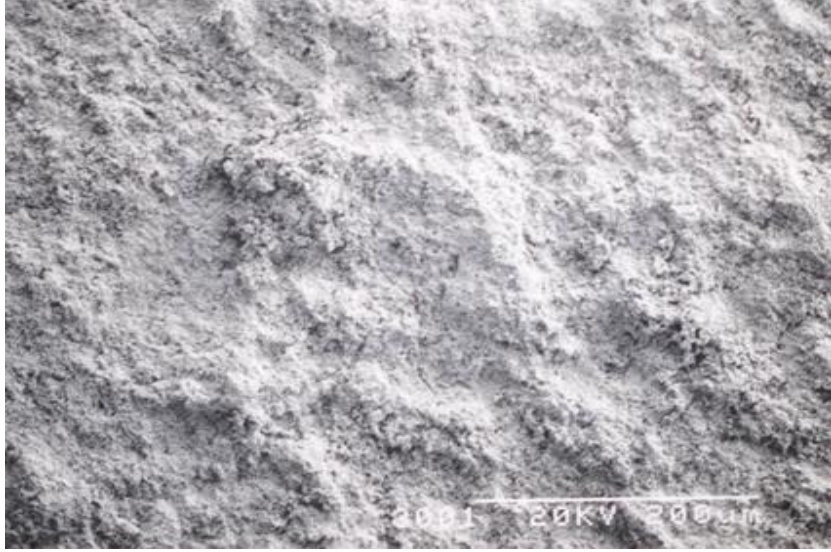
Figure 5.4: Photograph of molybdenum surface after a 6 kJ ET discharge showing surface ablation due to direct sublimation.
