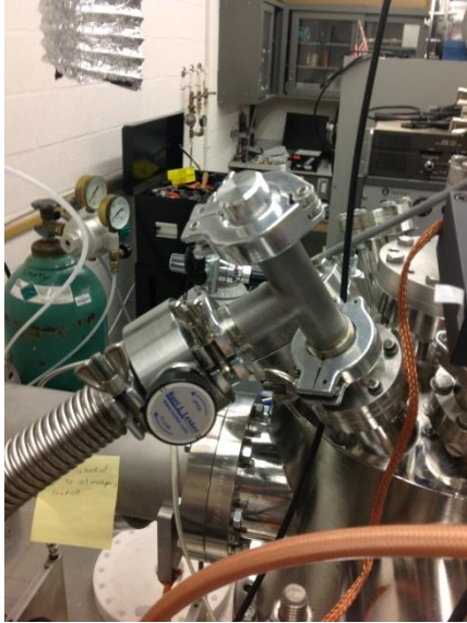
Figure 30: Pressure valve that connects vacuum chamber to rough pump only.
