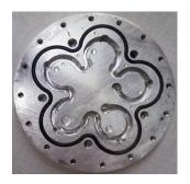
Figure 2.6: The center shows the flower patterned water channel surrounded by an O-ring and the holes for the bolts to hold it all together.
