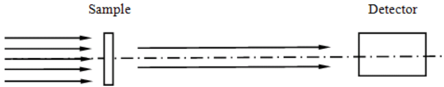
Figure 2.9: Principle of a transmission experiment.
