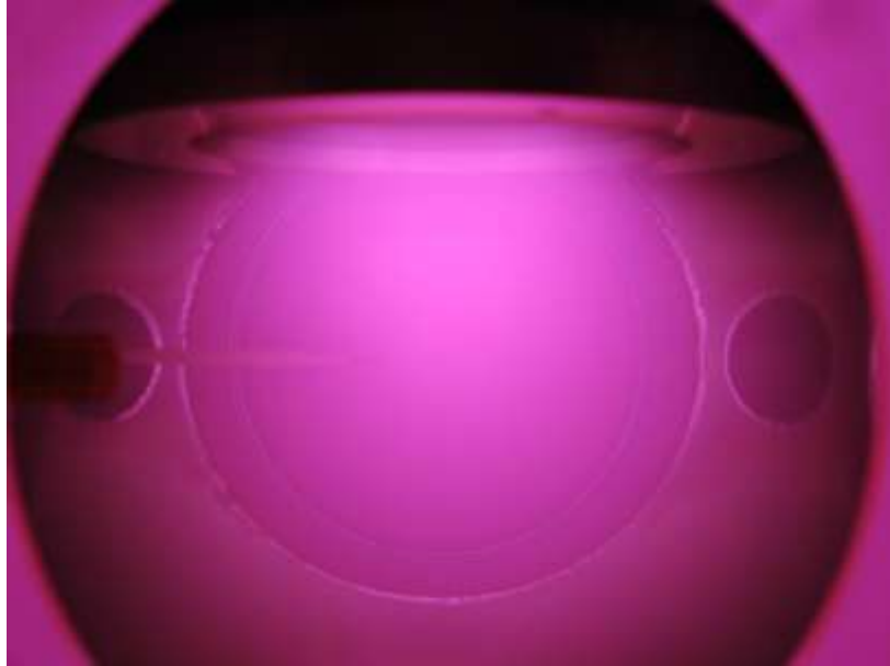
Figure 5.2. Modified GEC reference cell with top inductive electrode. The Langmuir probe (also pictured) is centered in the discharge approximately two inches from the quartz window on the top electrode.
