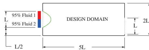
Fig. 2. The optimization model problem consists of two mixed fluids entering a channel to achieve mixing and exit through an offset outlet.
