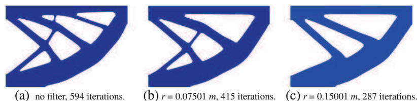
Fig. 12 Effect of filter radius on the optimized design for p = 0.2
