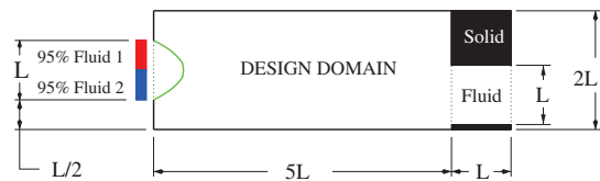
Fig. 4. Optimization model problem "Option B" augments "Option A" with a non-design region at the outlet.
