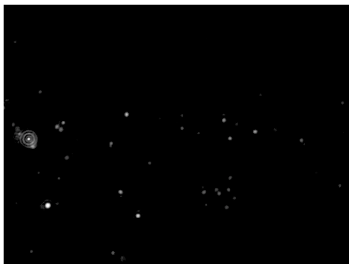
Figure 3.13: A screenshot from the NTA raw video output of egg-SM vesicles. Image approximately 120 \mu\text{m} x 90 \mu\text{m} .
