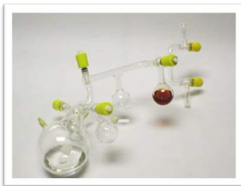
Figure 2.15 Living anionic polymerisation reaction vessel called 'christmas tree'.
