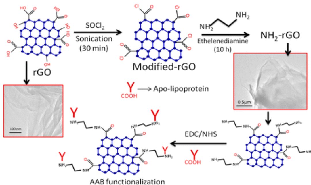
Figure 7-26: Apo-lipoprotein B 100 functionalisation on an NH 2 -rGO sheet for LDL detection. Reprinted with permission from [467]. Copyright (2014) American Chemical Society.
