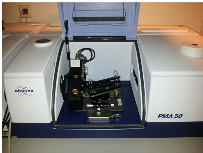
Figure 54. Bruker Vertex 80 fitted with a PMA 50 modulation unit, used for PM-IRRAS.
