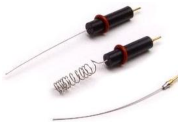
Fig. 5. Different shape of platinum pseudo-reference electrode.
