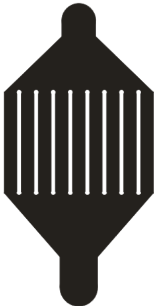
Fig. 83. SU8-50 microfluidic channels mask.
