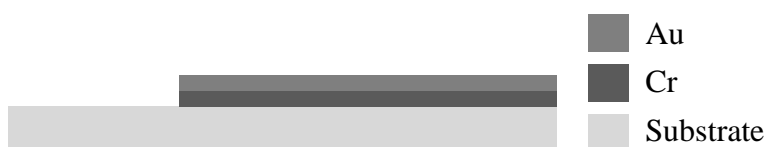
Fig. 80. Cross section diagram of the substrate covered with Cr and Au.
