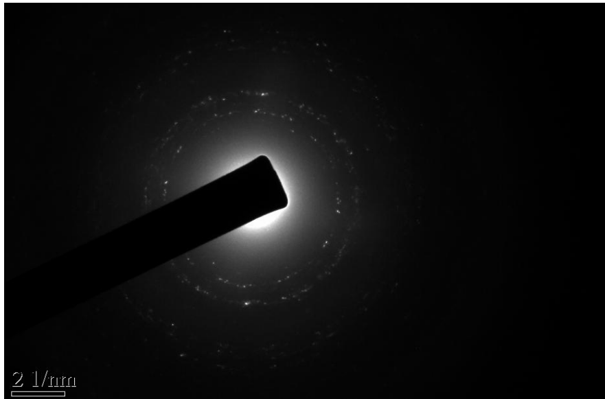
Figure 84 b): Electron diffraction pattern obtained from the bright field image in Figure 84 a).
