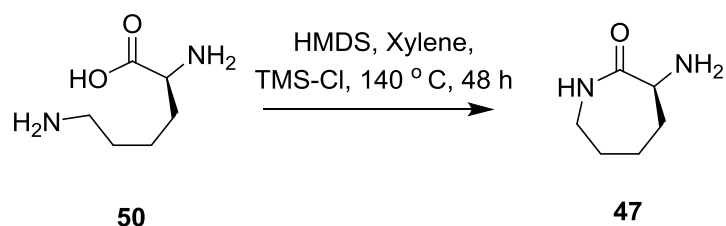
Scheme 5.3 Non-racemising cyclisation of D-lysine ( 50 ) to form D- \alpha -amino- \epsilon -caprolactam ( 47 ) (Attempted previously in Cobb group by S. Maddrell, 2009.)
