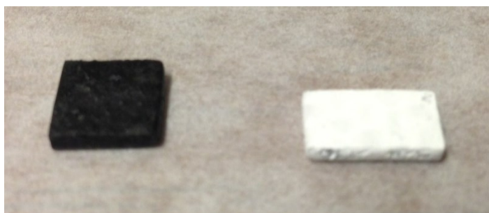
Fig. 92. SiCN-HfO 2 infiltrated SiC preform before (left) and after (right) oxidation
