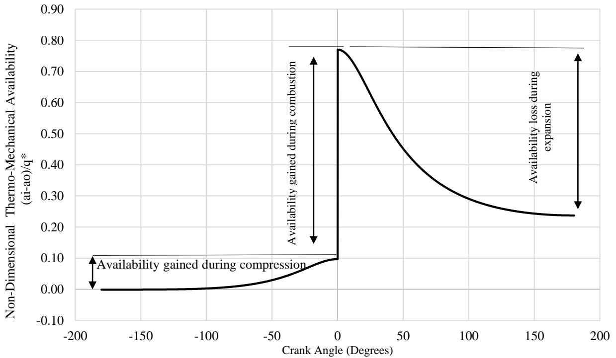
Figure 31. The non-dimensional thermo-mechanical availability versus crank angle for the ideal Otto cycle using methane at an equivalence ratio of 1.
