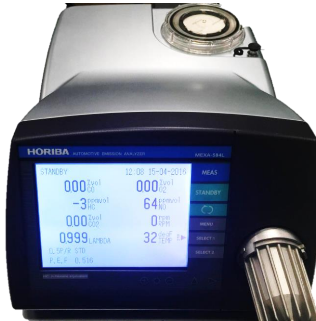
Figure 10. Exhaust gas analyzer (model MEXA-584L) used in the current experiment.
