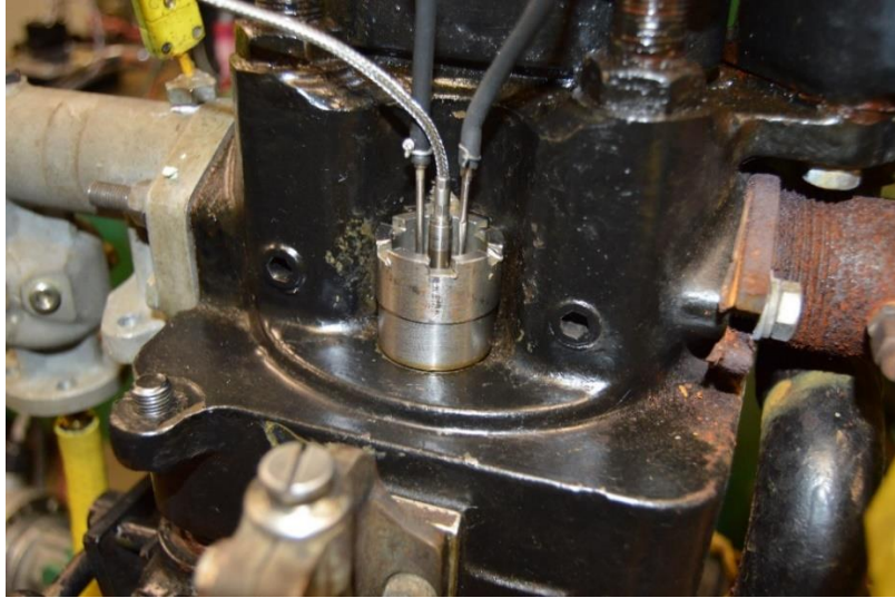
Figure 8. The in-cylinder water-cooled pressure transducer (Kistler model 7061B).
