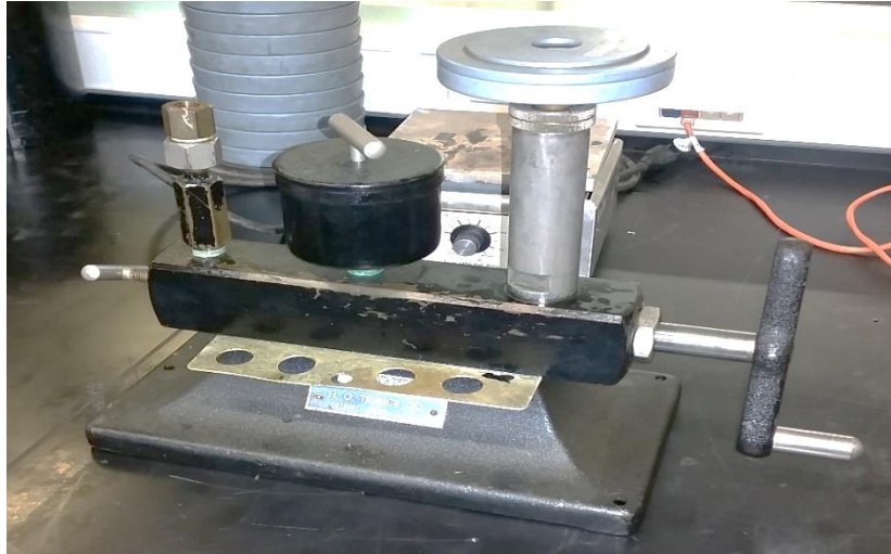
Figure 12. Dead-weight-tester used for static calibration of the fuel pressure sensor.
