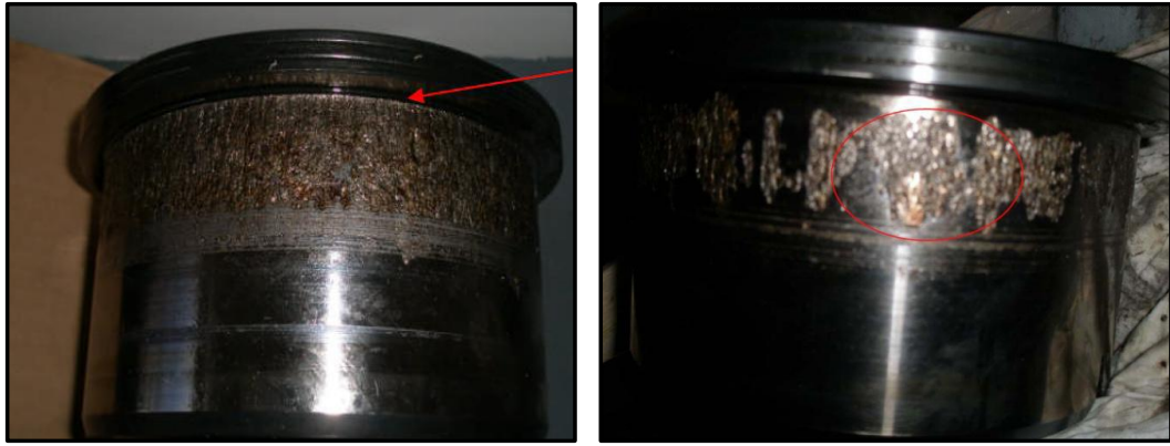
Figure 39: Damaged intermediate shaft bearing inner races of (a) Turbine X and (b) Turbine Y
