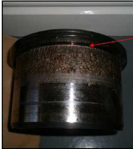
Figure 32: Turbine X intermediate shaft bearing inner race under inspection following its replacement
