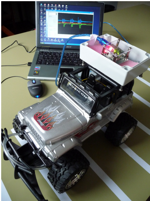
(a) A radio-controlled vehicle carrying an accelerometer is used for simulating the robot behavior inside the pipeline.
