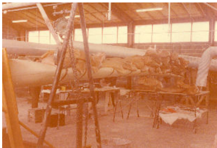
Figure 2.1- Static blade tests using sandbags, 1978 and 1981 [89]
