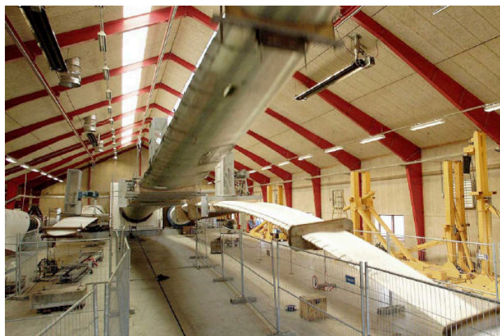
Figure 2.5 - Resonant testing using rotating eccentric mass at Sparkær [93]
