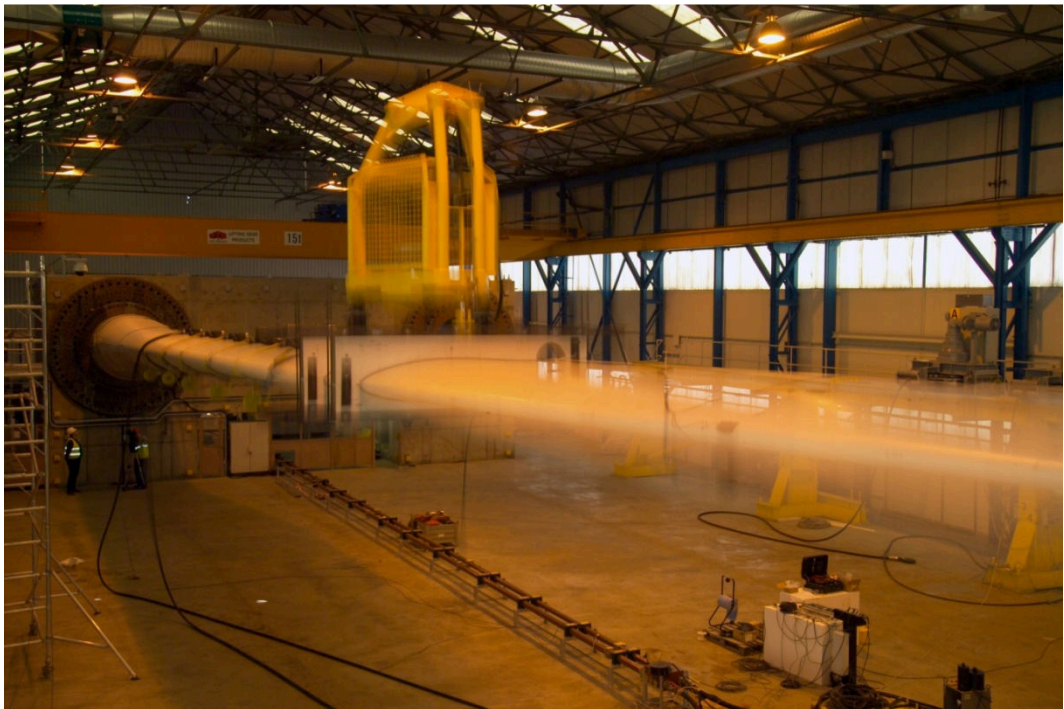
Figure 1.13 - Single axis resonant fatigue test
