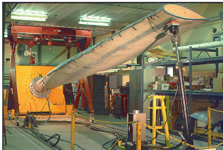
Figure 2.3 – Single point forced displacement testing at NREL, USA [18]
