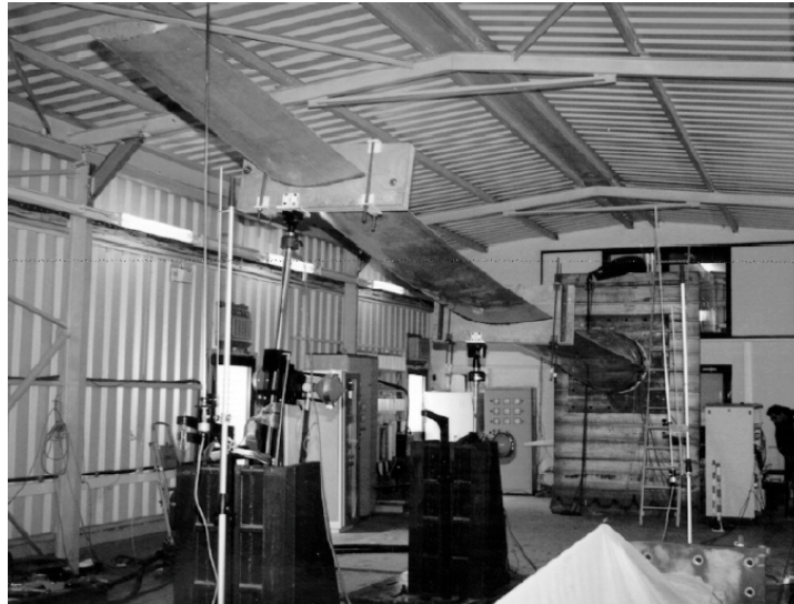
Figure 2.4 - Forced displacement testing with multi point loading at CRES, Greece [18]
