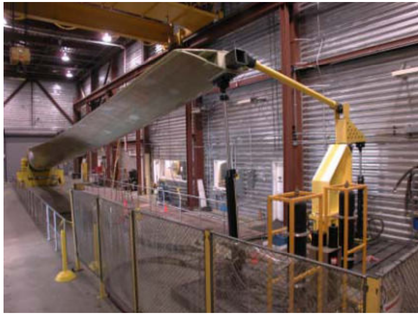
Figure 1.12 - Dual axis forced displacement testing
