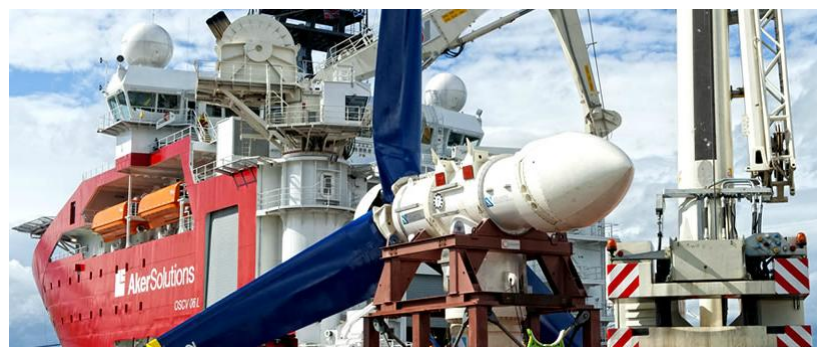
Figure 3.13 AR series horizontal axis turbine on fixed support tower
