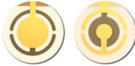
Grey=quartz, yellow=metallic gold electrodes. Front side (left), Back side (right)
