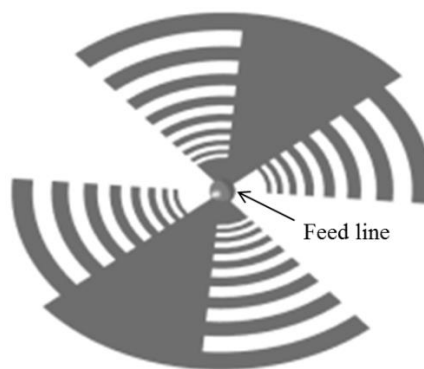
Figure 3.9 – A typical log-periodic antenna (adapted from [24]).
