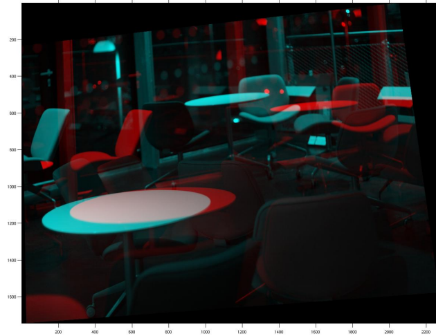
Figure 7.7: The Result obtained from Rectifying The Images using Data Obtained from the Orientation Sensor
