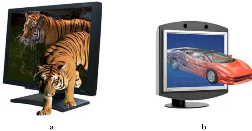
Figure 2.6: Examples of autostereoscopic 3D displays: DTI Virtual Window 19 (a) and SeeReal C-i display with head tracker (b). [From http://www.inition.co.uk , last accessed: 11.07.2011].
