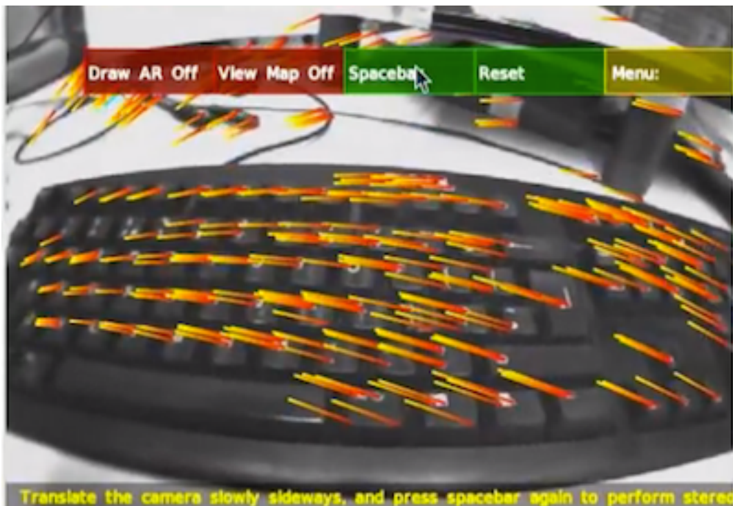
Figure 2.4: Lateral Translation for Stereo Initialisation in PTAM
