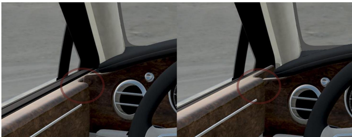
Figure 1- Movement of the door where it meets the dashboard, creating significant variation and inconsistency in the design
