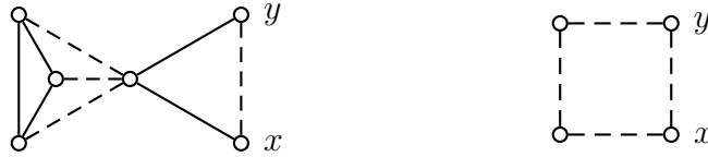
Figure 4.5: Strong negators: the dashed lines represent blue negators in the left graph and red negators in the right. Their endpoints are the vertices x and y from these negators.
