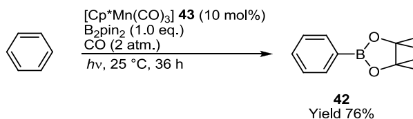
Figure 6 - The photocatalysed borylation of benzene with [\text{Cp}^*\text{Mn}(\text{CO})_3] .
