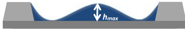
Figure 4.8: A schematic diagram showing the definition of h_{max} for solvents which dry to give a W-shaped film profile.
