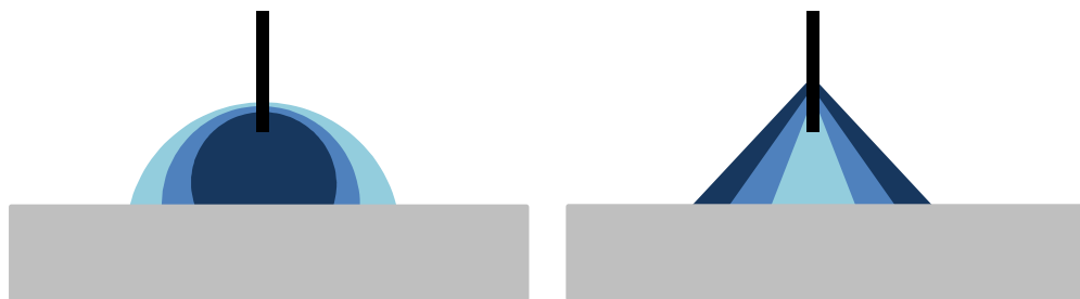
Figure 2.15: Schematic diagrams showing the measurement of advancing (left) and receding (right) contact angles. The darkest blue shade represents the earliest time in measurement with the lightest blue representing the latest time in measurement.
