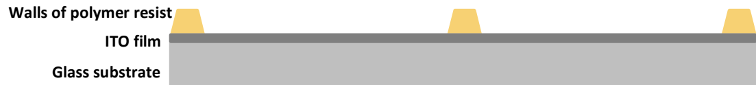
Figure 2.12: A schematic diagram showing the different layers present in the substrates. Not to scale.
