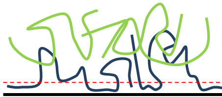
Figure 2.7: Sketch of the polymer layers near a filler surface; red line is the boundary of the restricted layer, blue chains are bound to the surface, green chains are unbound
