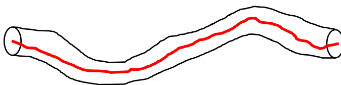
Figure 2.2: Visual of reptation model, polymer chain (red) trapped in a reptation tube (black)
