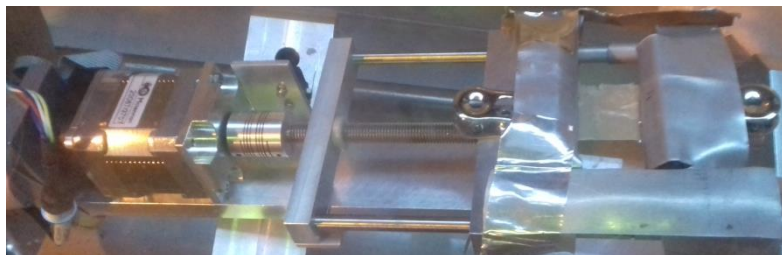
Figure 3.19: Image of neutron scattering strain rig including driving motor and cadmium shielding, IRIS workstation
