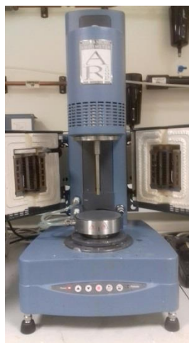
Figure 3.11: AR2000 rheometer with peltier stage and 8 mm head attached
